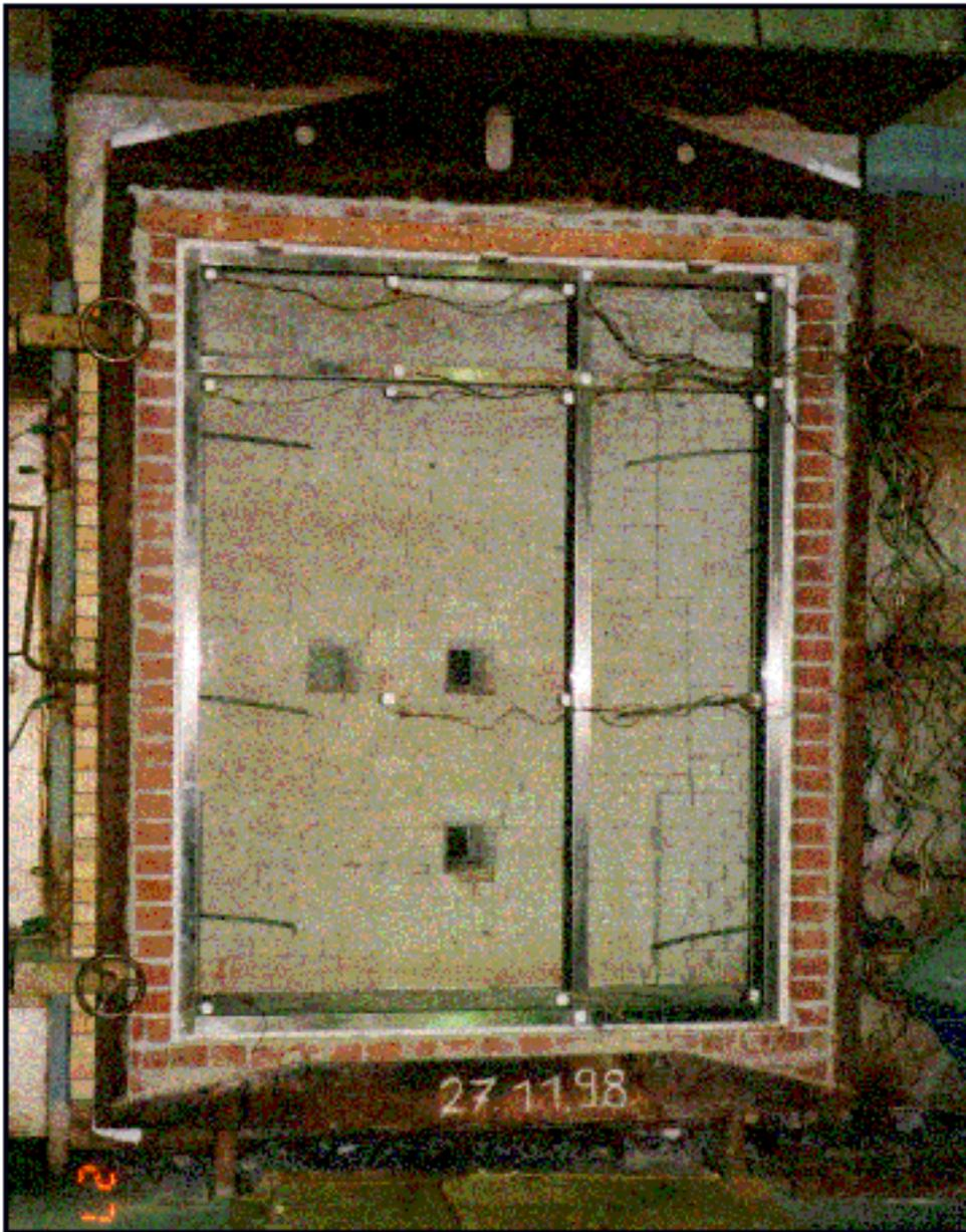
*Fig.1. Glazed element mounted in front of an oven for fire tests*
